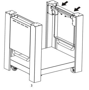
5. Assembly body and cart by using a L shape sheet from outside.
